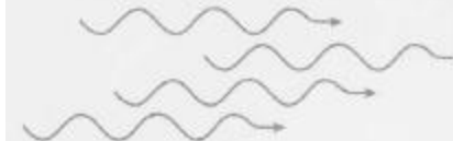
Figure 9.21 Coherent versus incoherent light.
