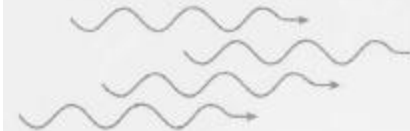
Figure 9.21 Coherent versus incoherent light.
